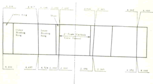
FIG. 6. Cross section of binding ring set giving diametral dimensions. The rings are assembled from the outside to inside. The 2.485-in./2.365-in. surface is finished after B-C-D are pressed in place. The shim ring is split axially into four pieces for ease of removal of broken dies. Small adjustments in the interference of the core in the rings may be made with thin steel shim stock wrapped around the core vessel.
